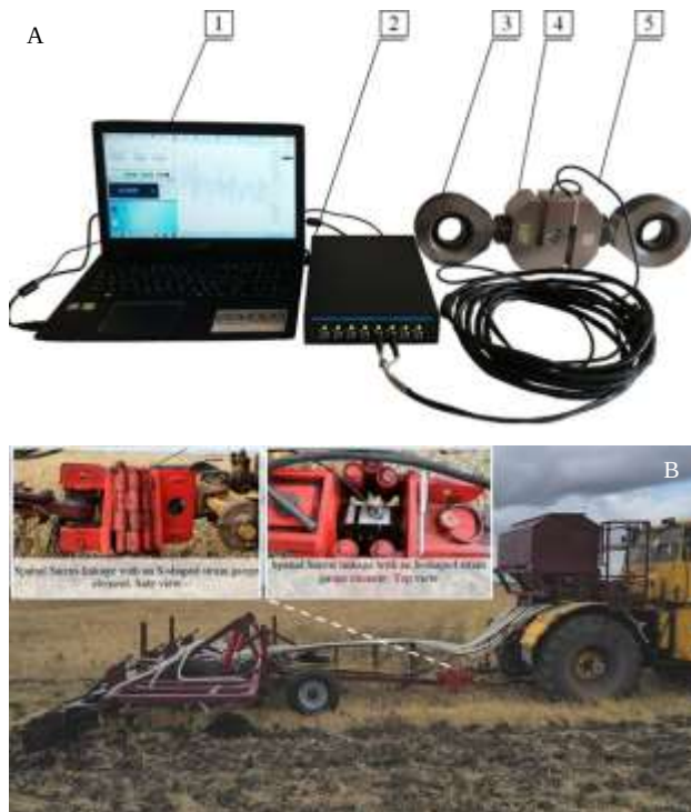
Fig. 3: Strain gauge equipment used in experimental studies; 1. Personal computer; 2. Strain gauge system; 3. Force-transmitting devices; 4. Force sensor; 5. Shielded wire ; a) Exterior view of the strain gauge equipment; b) Components of the strain gauge equipment installed on the tractor's hitch system.
