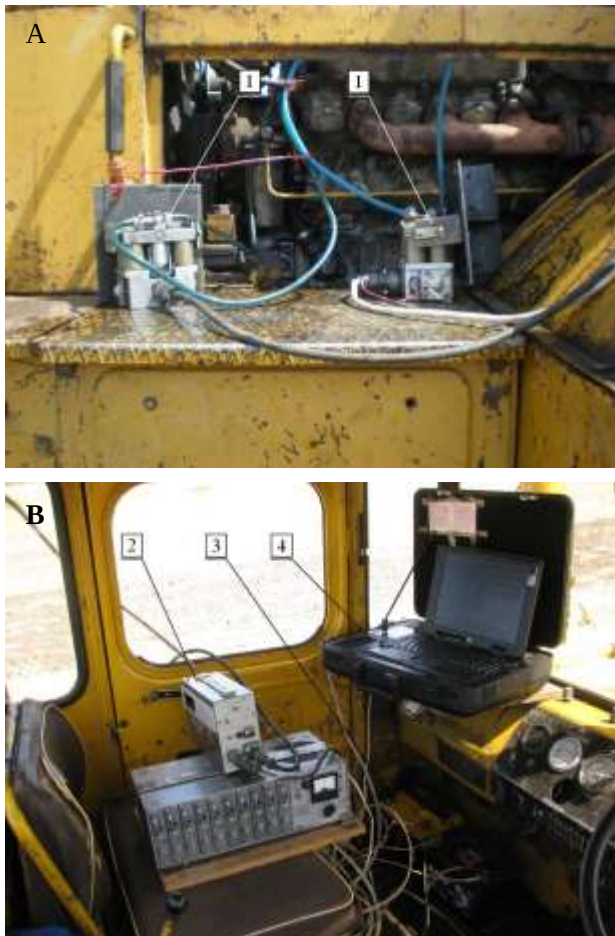
Fig. 5: IP-197 fuel meter with IP-238 information-measurement system; 1 – fuel flow sensor; 2 – fuel meter electronic unit; 3 – accumulator battery; 4 – IP-238 information-measurement system; a) fuel flow sensors installed in the tractor's fuel system; b) fuel meter components installed in the tractor cabin.
