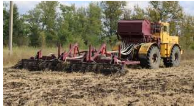
Fig. 6: The cultivator-fertilizer prototype coupled with the K-701 tractor while performing the technological process.
