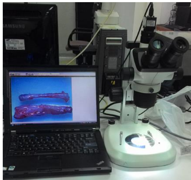
Fig. 1: The stereo dissecting microscope alone PC used for bone length measurement.
