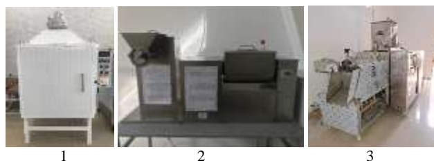
Fig. 2: The apparatus used for the study: 1 - drying oven; 2 - laboratory mixer; 3 - twin-screw extruder (SYSLG 32).
