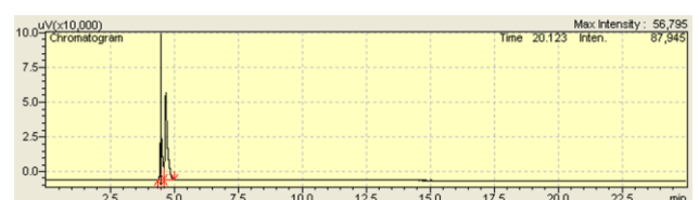
Fig. 4b: Chromatogram of 5% ethanol and 1% methanol (control solution).
