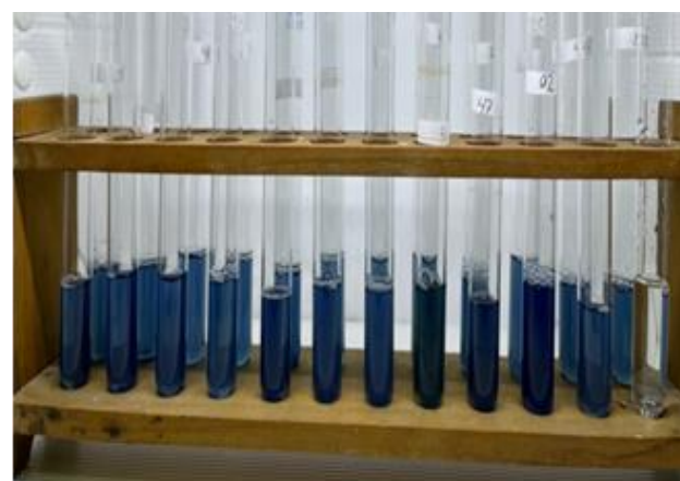
Fig. 2: Qualitative analysis of dissolved phosphate using liquid Pikovskaya medium with the addition of 0.5 mL concentrated ammonium molybdate and potassium antimonyl tartrate blue reagent.
