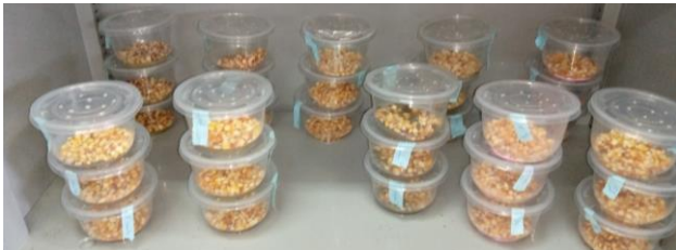
Fig. 2: Plant powders ( Calotropis procera and Cassia siamea ) and pesticide Actellic 2% DP® mixed with the 50 g maize seeds
