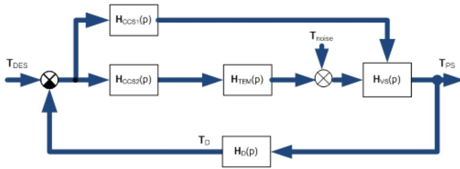
Fig. 2: Functional model of an energy-saving trigenerative climate management system.
