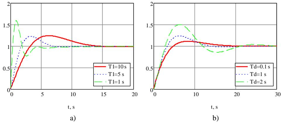
Fig. 3: Dynamic response of the system with various time constants of TEM (a) and climate detector (b).
