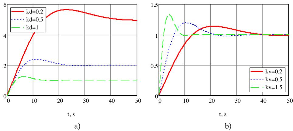
Fig. 4: Dynamic response of the system with various gain of the climate detector (a) and ventilation system (b).
