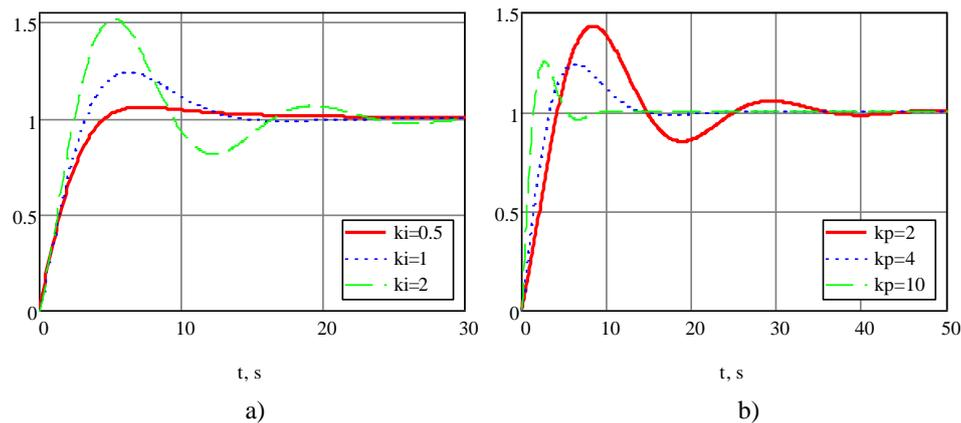
Fig. 5: Dynamic response of the system with various coefficients of inertia (a) and proportionality (b) of CCS2.
