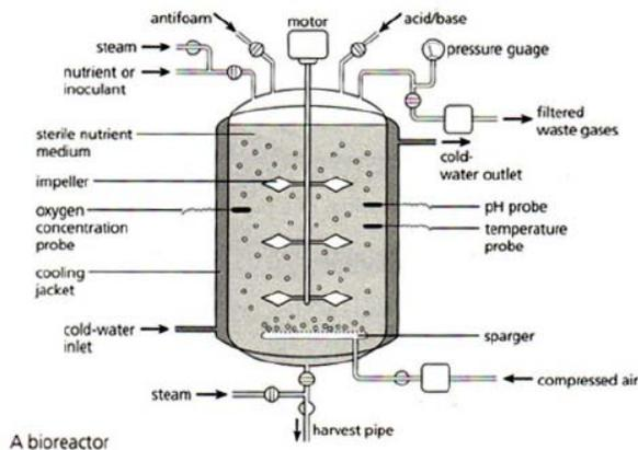
**Mixing:** In a bio reaction is achieved by stirrers or pumps, resulting in a turbulent current.
