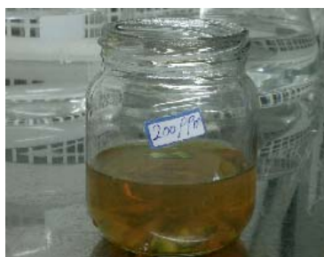
Fig. 2: Explants were submerged in 200 ppm Nano-silver solution.
