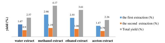
Fig. 1: The yield of the first extraction, the second and the total yield from the *Manilkarazapota* bark with water, methanol, ethanol and acetone as the solvent agents.
