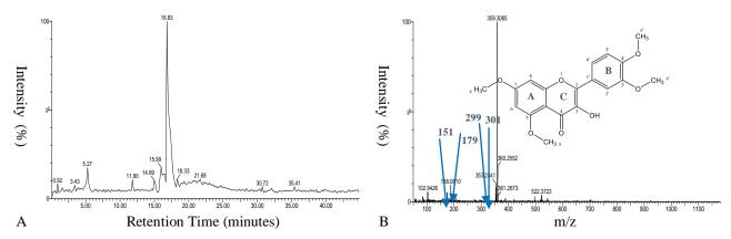
Fig. 2: The chromatogram of TF methanol fraction (A) and the peak of mass sprectum compound on minute 16.83 in chromatogram of TF methanol fraction (B).
