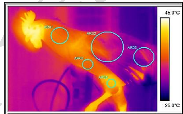
Fig. 2: Visualization of the body area temperature of chickens using the infrared thermography (IRT).
